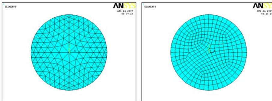
**Fig. 4** Piecewise linear basis function on 2D domain discretized by triangles and bilinear basis function on 2D domain discretized by squares
