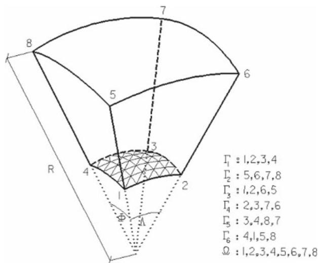
**Fig. 1** Illustration of the computational domain, the Earth's surface  $\Gamma_1$  is approximated by series of triangles
