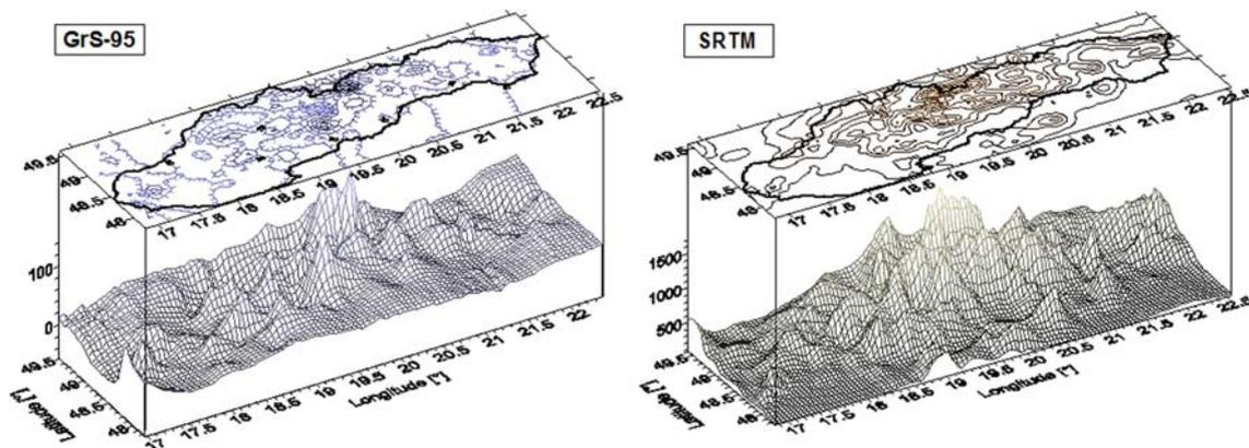
**Fig. 8** Surface gravity disturbances computed from detailed gravimetric mapping GrS-95 and the terrain topography in Slovakia
