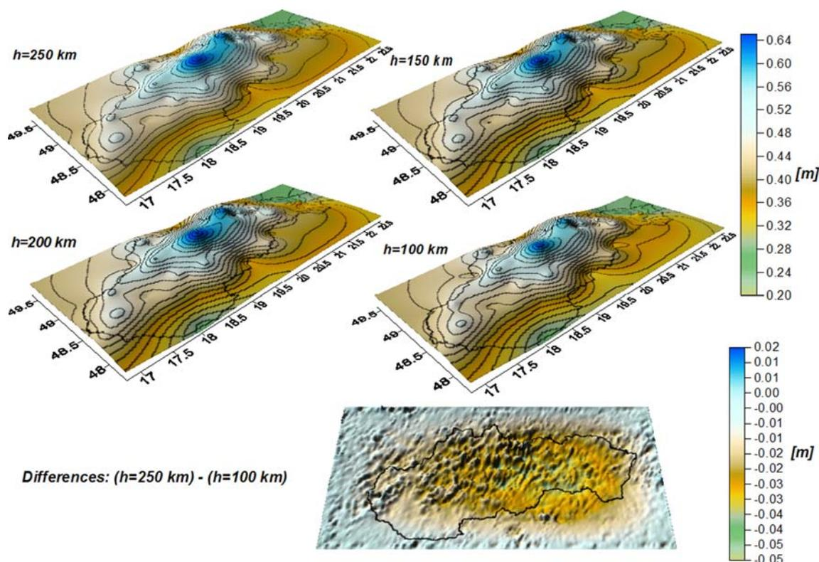
**Fig. 10** Differences between the FEM solutions and the GPS/levelling method with 5 km discretization and the height of the upper boundary: 100, 150, 200 and 250 km
