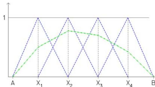
**Fig. 2** Discretization of 1D domain, basis functions  $v_i$  (blue dashed lines) and their linear combination (green dot-and-dash line) that is piecewise linear
