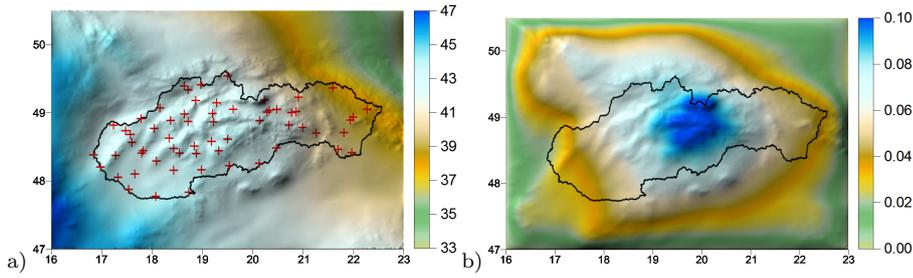
**Fig. 3** a) Quasigeoidal heights  $\zeta[m]$  obtained by solving the NSFGBVP, b) Differences in  $\zeta[m]$  between  $10^{th}$  and  $1^{st}$  iteration. Red crosses denote the distribution of 61 GPS/levelling points.
