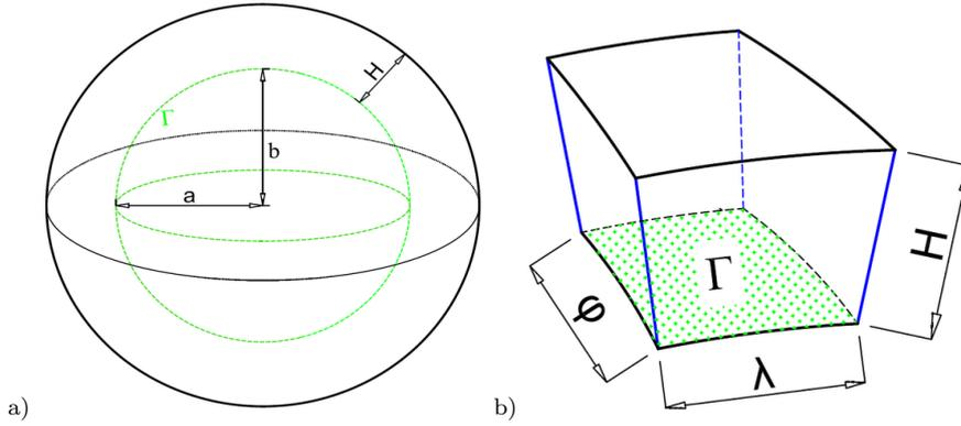
**Fig. 1** Sketch of the computational domain  $\Omega$  for a) global numerical experiment, b) local numerical experiment. The dotted boundary  $\Gamma$  represents the part of the Earth's surface,  $\varphi$  and  $\lambda$  denote latitude and longitude and  $H$  denotes the height above WGS84.
